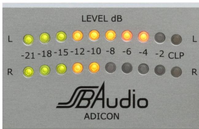
With the VU meters, customary in tape recorders, it is totally different: There is no distinct limit on tape recorders. With a rising level only the harmonic distortions increase moderately, so that overdriving, particularly at short peaks, hardly carries any weight. Full scale in tape recorders depends more on the trade-off between dynamic range and distortion and is, in contrast to the level control of digital signals, relatively arbitrary.
