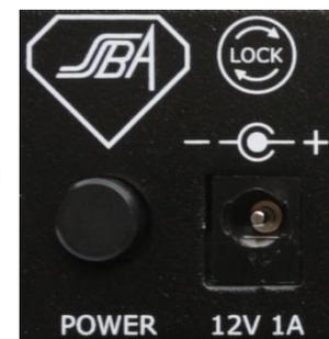
The ADICON is turned on by pressing the **POWER** switch. The operation is indicated by the illumination of one of the two LEDs **SOURCE** on the front panel.
